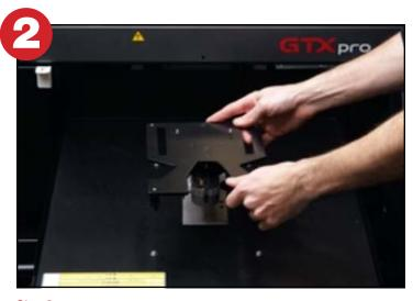
**Step 2:**Insert the T-Lock Base into the platen stem of the Brother DTG printer.
