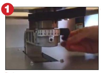
**Step 1:**Remove the Adult Platen by loosening the Locking Lever and lifting the platen straight up.
