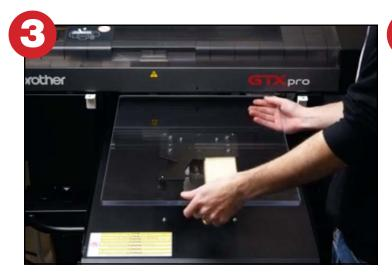
**Step 3:**Install the T-Lock XL Insert so T-Lock brackets slide into the slots in T-Lock Base.
